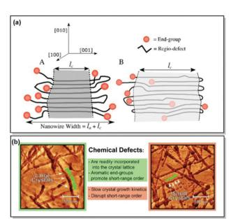
Fig. 3 (a) Proposed P3HT nanowire structures with (A) complete or (B) partial defect expulsion, where the darker grey area corresponds to the higher crystallinity region. (b) Young's modulus AFM scans of P3HT nanowires with lower (left panel) and higher (right panel) defect concentration. Reproduced with permission from American Chemical Society. 70
