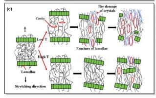
Fig. 1 (a) Microstructural features in CPs. Reproduced with permission from Wiley.<sup>25</sup> (b) Morphological changes along with associated hole and ion transport in PEDOT:PSS (Scheme 1). The arrows correspond to the intracrystalline hole transport. Reproduced with permission from Springer Nature.<sup>26</sup> (c) Strain-induced microstructural changes in a semicrystalline polymer. Reproduced with permission from Elsevier.<sup>27</sup>
