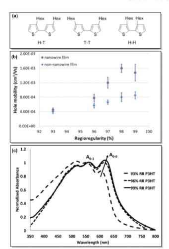
**Fig. 2** (a) Possible coupling products of **P3HT** (H–T: head-to-tail, T–T: tail-to-tail, H–H: head-to-head). (b) Correlation between RR and hole mobility for **P3HT** nanowire and non-nanowire films. (c) UV-Vis absorption spectra for **P3HT** with various RR%. Reproduced with permission from American Chemical Society. <sup>67</sup>
