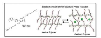
Fig. 8 Chemical structure of PB2T-TEG along with the uncovered unzipping/zipping mechanism for ion insertion. Reproduced with permission from American Chemical Society.83
