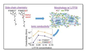
Fig. 6 Top-left panel: chemical structures of P3MEET and P3MEEMT. Top-right panel: Schematic representation of LiTFSI distribution within P3MEET/P3MEEMT semicrystalline structure at high concentration of LiTFSI. Bottom panel: P3MEET and P3MEEMT ionic conductivity at 90  $^{\circ}$ C. Reproduced with permission from American Chemical Society.  $^{81}$
