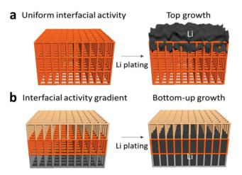
Fig. 10 Growth of lithium metal on the framework with (a) uniform interfacial activity and (b) interfacial activity gradient. The figures are reproduced from ref. 231.227
