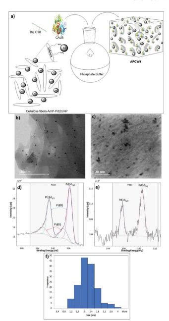
Fig. 2 (a) Fabrication of APCW9. STEM images of APCW9, (b) scale bar 100 nm and (c) scale bar 20 nm. XPS spectra of Pd 3d5/2 for (d) MCC-Amp-Pd<sup>0</sup> and (e) APCW9 (that had been stirred for 24 h in toluene, at 90 °C, under H<sub>2</sub> atmosphere). (f) Size distribution of the Pd nanoparticles of APCW9
