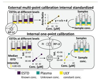
**Fig. 1** The two combined quantification strategies: (1) external multipoint calibration with internal standardization and (2) internal one-point calibration. LILY (yellow) was added to the plasma sample (blue) and the ESTDs (purple) in the same concentration. ESTDs were measured *via* RP-LC-HRMS and FI-HRMS. Samples were only measured *via* RP-LC-HRMS
