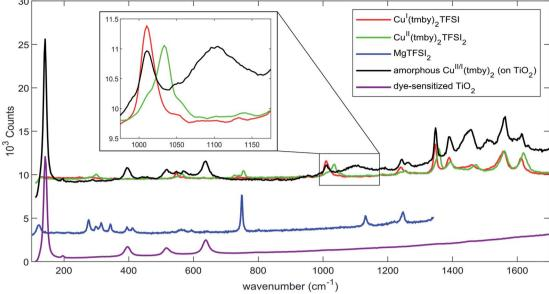
Fig. 4 Raman spectra of  $Cu^{II/I}(tmby)_2$  TFSI<sub>(2)</sub> and MgTFSI<sub>2</sub> (powders), DSCs sensitized with the XY1:L1 sensitizer combination as well as (sensitized) DSCs containing amorphous  $Cu^{II/I}(tmby)_2$  TFSI<sub>(2)</sub> hole transport material. The two latter spectra were recorded inside the 'sandwich' DSC. Spectra are offset for clarity.
