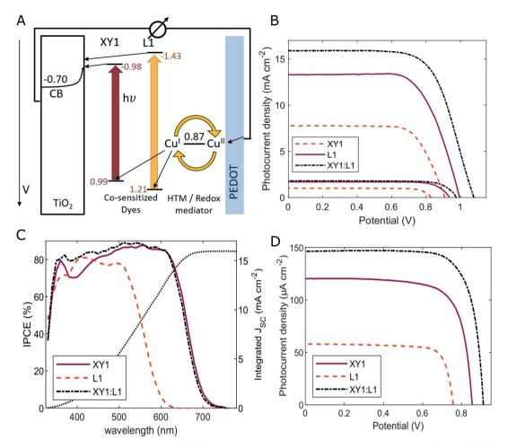
Fig. 2 (A) Working principle of the XY1:L1-sensitized DSC. (B) Photovoltaic performance under simulated sunlight (AM 1.5G, 100 mW cm<sup>-2</sup>) and 10% sunlight, (C) incident photon to current conversion efficiency spectra (IPCE), and (D) photovoltaic performance under 1000 lux fluorescent light (303.1  $\mu$ W cm<sup>-2</sup>) of XY1, L1 and XY1:L1 co-sensitized DSCs. Corresponding parameters are listed in Table 1.
