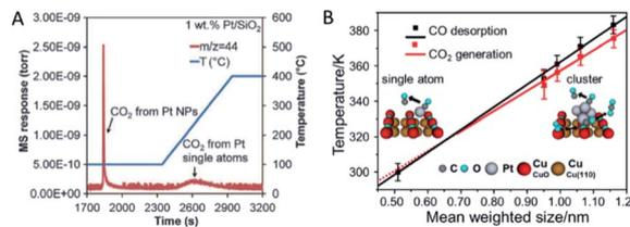
Fig. 6 (A) CO<sub>2</sub> signal monitored by the mass spectrum during the temperature-programmed oxidation process of the pre-adsorbed CO on Pt/SiO<sub>2</sub>. Reproduced with permission.<sup>73</sup> Copyright 2015, American Association for the Advancement of Science. (B) Plots of the CO desorption and CO<sub>2</sub> generation temperatures *versus* the mean size of the Pt nanoclusters. Reproduced with permission.<sup>13</sup> Copyright 2016, American Chemical Society.
