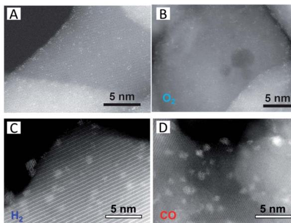
Fig. 2 (A) HAADF-STEM images of the as-prepared 1.66 wt% Pt<sub>1</sub>/Fe<sub>2</sub>O<sub>3</sub> SAC and the samples treated in (B) O<sub>2</sub>, (C) H<sub>2</sub>, and (D) CO at 250 °C for 2 h. Reproduced with permission.<sup>50</sup> Copyright 2018, IOP Publishing Ltd.
