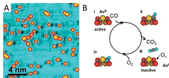
Fig. 4 CO oxidation catalysed by Au single atoms on the CuO monolayer. (A) STM image of the Au single atoms exposed to CO at RT. (B) Schematic illustration of the CO oxidation process activated by the Au single atoms on the CuO monolayer. Reproduced with permission.<sup>56</sup> Copyright 2018, American Chemical Society.
