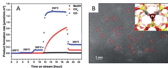
Fig. 7 (A) Product formation rate on the  $\text{Ni}_x\text{Mg}_{1-x}\text{O}$  samples at different temperatures. Reproduced with permission.<sup>49</sup> Copyright 2019, American Chemical Society. (B) STEM-HAADF image of the catalyst after the reaction, with the inset showing the computational model of the single iron atom bonded to two C atoms and one Si within the silica matrix. Reproduced with permission<sup>15</sup> Copyright 2014, American Association for the Advancement of Science.
