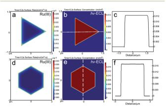
Fig. 3 Results of the simulated reaction rate and concentration profiles. The generation rate of Ru(III) on the gold (a) triangular and (d) hexagonal nanoplates. The ECL spatial intensity distribution on the gold (b) triangular and (e) hexagonal nanoplates. (c and f) The distribution of ECL intensity at the measuring line marked in (b and e).
