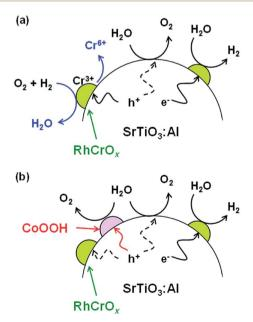
Fig. 3 Illustrations of (a) RhCrO<sub>x</sub>/SrTiO<sub>3</sub>:Al deactivation mechanism and (b) stabilisation of RhCrO<sub>x</sub>/SrTiO<sub>3</sub>:Al by CoOOH. The stoichiometry of the reactions is ignored for simplicity.
