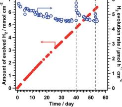
Fig. 4 Time course of water splitting activity of  $5 \times 5$  cm<sup>2</sup> TiO<sub>2</sub>/ CoOOH/RhCrOx/SrTiO3:Al sheet in panel reactor. Reaction conditions: photocatalyst, 20 mg; reaction solution, 1 mm deep distilled water; reaction temperature, 291 K; light source, AM 1.5G solar simulator. Asterisk symbols (\*) indicate interruption of the illumination for two days
