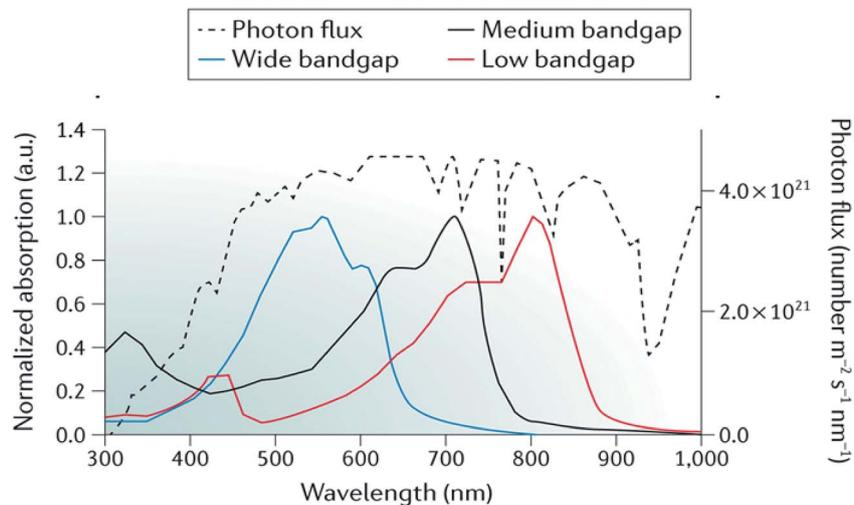
Fig. 10 Representative absorption spectra of wide-bandgap, medium-bandgap and low-bandgap donor polymers used in tandem organic solar cells alongside the AM 1.5G solar spectrum (black dotted curve). ICL, interconnecting layer; TCO, transparent conductive oxide. Adapted by permission from Springer Nature: Li *et al.*, *Nature Mater. Rev.*, Copyright 2017.<sup>97</sup>
