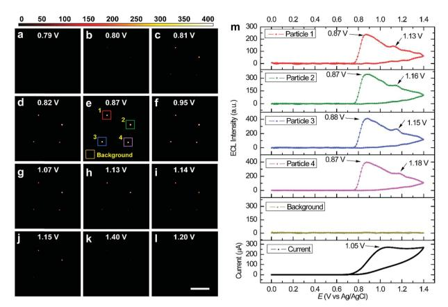
Fig. 2 (a–l) Successive ECL snapshots of four RuDSNs during a potential cycle. Scale bars (white), 30  $\mu$ m. (m) ECL intensity of four nanoparticles and blank area in (e) as a function of electrode potential and the corresponding CV curve of the GC electrode (black line) recorded by the potentiostat. The potential was cyclically scanned from 0 to 1.4 V at a scan rate of 20 mV s<sup>-1</sup> in 200 mM PBS buffer containing 100 mM TPA. The exposure time of EMCCD was 500 ms.
