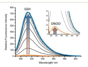
Fig. 1 Fluorescence spectra of GSH-PF3 (0.5  $\mu$ M) with addition of ONOO<sup>-</sup> (10  $\mu$ M) (inset) followed by the addition of GSH (0–80  $\mu$ M), 5 min wait between addition in buffer solution [52 wt% methanol] (pH = 8.21 at 25 °C). Fluorescence intensities were measured with  $\lambda_{ex}$  = 488 nm with slit widths ex slit: 5 nm and em slit: 2.5 nm.
