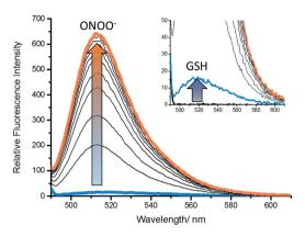
Fig. 2 Fluorescence spectra of GSH-PF3 (0.5 μM) with addition of GSH (200  $\mu$ M), 10 min wait (inset), then addition of ONOO<sup>-</sup> (0–10  $\mu$ M) in buffer solution [52 wt% methanol] (pH = 8.21 at 25 °C). Fluorescence intensities were measured with  $\lambda_{ex} = 488$  nm with slit widths ex slit: 5 nm and em slit: 2.5 nm.
