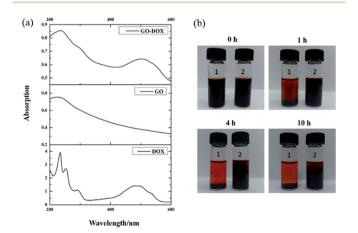
Fig. 3 The UV-vis spectra (a) of DOX, GO, and GO-DOX and the digital photos (b) for stability investigation of F127-GO-DOX hydrogel (sample 2) with GO-DOX (sample 1) solution as a control at different times
