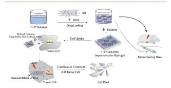
Scheme 1 Synthesis and mechanism of F127-GO-DOX supramolecular hydrogel system.
