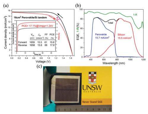
Fig. 8 (a) J-V curve and the steady-state PCE in the inset for the champion tandem device on 16 cm<sup>2</sup> using the heavier p++ front emitter for the Si bottom cell. (b) EQE for the corresponding tandem device (black), for the perovskite top cell (blue), and the silicon bottom cell (red). The total absorbance (1-reflectance) of the tandem device is shown by the green line. (c) A photo of a fabricated 16 cm<sup>2</sup> tandem.
