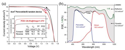
Fig. 7 (a) J-V curve and in the inset: steady-state PCE of the champion tandem device on 4 cm<sup>2</sup> using the heavier p++ front emitter for the Si bottom cell and with antireflection foil on the front of the tandem. (b) EQE for the corresponding device (black), for the perovskite top cell (blue), and for the silicon bottom cell (red). The total absorbance (1-reflectance) of the tandem device is shown by the green line.
