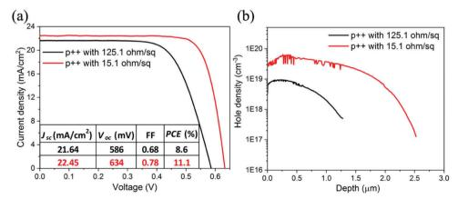
Fig. 4 (a) Current density-voltage (J-V) curves of Si bottom cells that have different p++ emitter profiles (black for 125.1 ohm sq<sup>-1</sup>). (b) Doping profiles of the same cells measured with electrochemical capacitance-voltage measurements.
