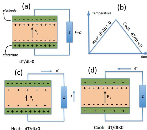
Fig. 3 The pyroelectric effect; (a) polarised material and corresponding surface charge (b) applied thermal cycle (c) heating leads to a decrease in polarisation and free surface charge for current generation (d) cooling leads to increase of polarisation leading to current reversal.
