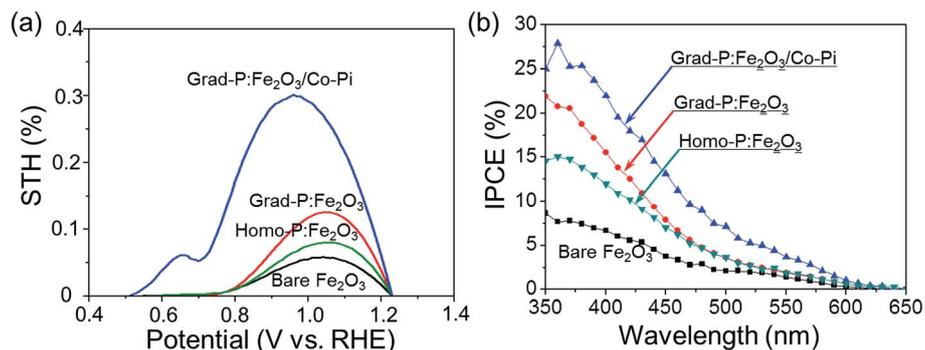
Fig. 9 (a) Photoconversion efficiency as a function of applied potential; (b) IPCE in the region 350–650 nm at a bias of 1.23 V (vs. RHE) for bare  $\text{Fe}_2\text{O}_3$ , homo-P: $\text{Fe}_2\text{O}_3$ , grad-P: $\text{Fe}_2\text{O}_3$  and grad-P: $\text{Fe}_2\text{O}_3/\text{Co-Pi}$  photoanodes.
