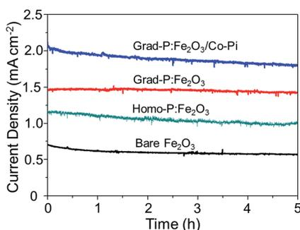
Fig. 10 Stability test of bare  $\text{Fe}_2\text{O}_3$ , homo-P: $\text{Fe}_2\text{O}_3$ , grad-P: $\text{Fe}_2\text{O}_3$  and grad-P: $\text{Fe}_2\text{O}_3/\text{Co-Pi}$  photoanodes for 5 h at 1.23 V (vs. RHE) under AM 1.5G illumination.
