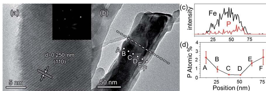
Fig. 2 (a) HRTEM image of a selected area of grad-P: $\text{Fe}_2\text{O}_3$ ; inset of (a) is the SAED pattern; (b) TEM image of a single grad-P: $\text{Fe}_2\text{O}_3$  bundle; (c) the P element distribution in a  $\text{Fe}_2\text{O}_3$  nanobundle (line in image b); (d) the P element concentration along the radial direction (dots in image b) (the error bar represents the standard deviation).
