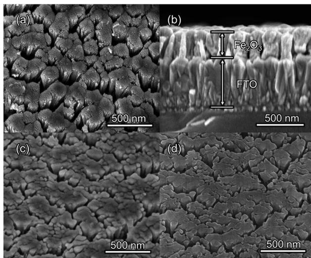
**Fig. 1** SEM images of (a) top-view and (b) side-view of bare  $\text{Fe}_2\text{O}_3$  (500 °C for 2 h); top-view of (c) bare  $\text{Fe}_2\text{O}_3$  (750 °C for 10 min after 500 °C for 2 h) and (d) grad-P: $\text{Fe}_2\text{O}_3$  (750 °C for 10 min after 500 °C for 2 h).
