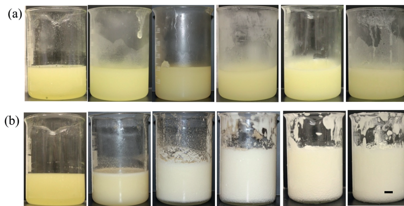
Fig. 5 Photographs of vessels containing mixtures of MA in HOSO at different concentrations (a) before aeration and (b) immediately (within 1 min) after whipping at 22 °C. MA concentrations in wt% are (left to right) 2.0, 3.5, 4.5, 5.0, 6.0 and 10.0. The sample at 2.0 wt% is one-phase, all other samples are two-phase. Scale bar = 1 cm.
