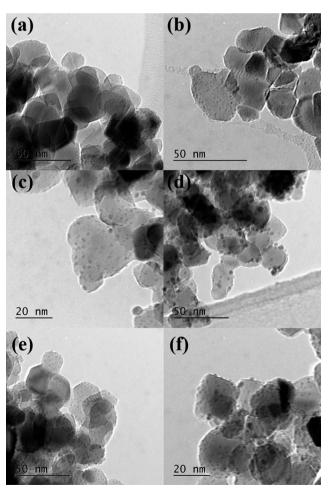
Fig. 3 TEM images of a) 4% Ru-1% Pd/TiO<sub>2</sub>; b) 3% Ru-2% Pd/TiO<sub>2</sub>; c) 2.5% Ru-2.5% Pd/TiO<sub>2</sub>, d) 2% Ru-3% Pd/TiO<sub>2</sub>; e) 1% Ru 4% Pd/TiO<sub>2</sub> and f) 0.5% Ru-4.5% Pd/TiO<sub>2</sub>
