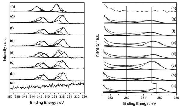
Fig. 6 XPS profiles of Pd(3d) and Ru(3d) core-level spectra of TiO<sub>2</sub> supported Pd with different Pd: Ru ratios. (a) 5% Ru/TiO<sub>2</sub>, (b) 4% Ru-1% Pd/ TiO<sub>2</sub>, (c) 3% Ru-2% Pd/TiO<sub>2</sub>, (d) 2.5% Ru-2.5% Pd/TiO<sub>2</sub>, (e) 2% Ru-3% Pd/TiO<sub>2</sub>, (f) 1% Ru-4% Pd/TiO<sub>2</sub>, (g) 0.5% Ru-4.5% Pd/TiO<sub>2</sub>, (h) 5% Pd/TiO<sub>2</sub>.
