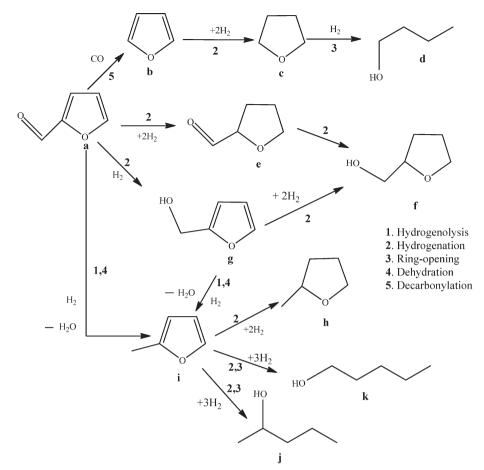
Scheme 1 Reaction pathways for FFR hydrogenation. Key: a. Furfural (FFR), b. Furan (F), c. Tetrahydrofuran (THF), d. Butanol (BuOH), e. Tetrahydrofurfural (THFF), f. Tetrahydrofurfuryl alcohol (THFA), g. Furfuryl alcohol (FA), h. 2-Methyltetrahydrofuran (2-MTHF), i. 2-Methylfuran (2-MF), j. 2-Pentanol (2-PeOH), k. 1-Pentanol (1-PeOH).
