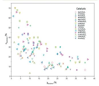
Fig. 1 Summary plot showing the percentage total selectivity for butenes vs. the percentage conversion of n-butane for catalysts 1-15 under condition sets A-H.
