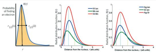
Fig. 2 Graphs showing a typical radial distribution function (RDF) based on the Slater-type orbitals used for deriving the four descriptors for (mixed) oxides (left), and examples of these orbitals for  $AgO_x$ :  $SrO_x/Al_2O_3$  (catalyst 1) and  $WO_x$ :  $MnO_x/Al_2O_3$  (catalyst 12).
