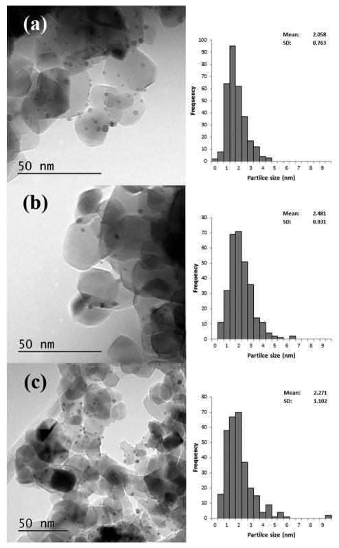
Fig. 4 Representative TEM images and associated particle size distributions for 1% Au/TiO<sub>2</sub> prepared by SIM a) no treatment, b) calcined at 250 °C and c) refluxed. Particle size distributions based on 300 particles.
