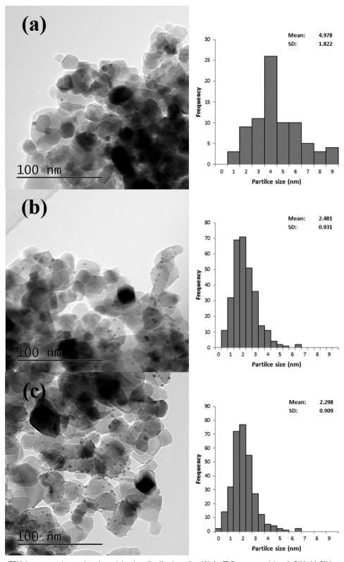
Fig. 2 Representative TEM images and associated particle size distributions for 1% Au/TiO<sub>2</sub> prepared by a) CIM, b) SIM and c) DP. Particle size distributions based on 300 particles.
