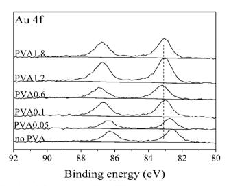
Fig. 8 Au(4f) spectra for 1% Au/TiO<sub>2</sub> SIM samples prepared with different ratio of PVA to Au (w/w).
