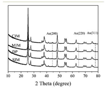
Fig. 1 XRD pattern of 1% Au/TiO<sub>2</sub> catalysts prepared with different methods
