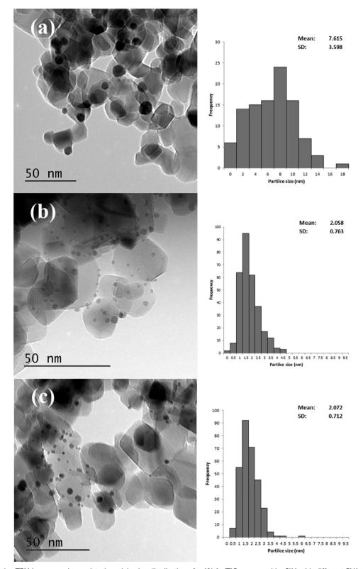
Fig. 9 Representative TEM images and associated particle size distributions for 1% Au/TiO<sub>2</sub> prepared by SIM with different PVA: Au ratios a) 0.1, b) 1.2 and c) 1.8. Particle size distributions based on 300 particles except for a) where 100 particles were counted.
