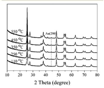
Fig. 5 XRD patterns of 1% Au/TiO<sub>2</sub> catalysts calcined at different temperatures.
