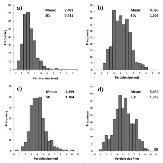
Fig. 7 Particle size distribution for % Au/TiO<sub>2</sub> SIM calcined at a) 250 °C, b) 350 °C, c) 450 °C and d) 550 °C.
