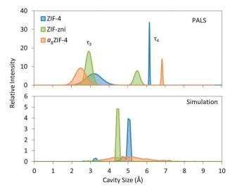
Fig. 2 Pore size distributions measured with PALS and simulated with  $Zeo++^{24,25}$  for ZIF-4, ZIF-zni and  $a_g$ ZIF-4. PALS results for the third and fourth components ( $\tau_3$  and  $\tau_4$ ) are represented as Gaussian distributions which correspond to the small and large cavities, respectively.
