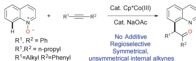
Scheme 1 Co(III) catalyzed C–H activation/oxygen atom transfer process.
