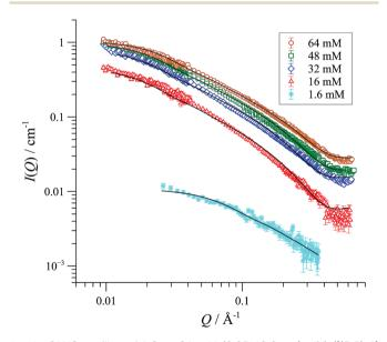
Fig. 2 SANS profiles of 1.6 to 64 mM (0.25-10.0 wt/vol%) {[(R,R)-1] [BArF]} $_n$  in THF-D $_8$ , 25 °C;  $_1(Q)$  = scattered intensity,  $_2(R)^{-1}$  = momentum transfer =  $_3(R)^{-1}$  = momentum transfer =  $_3(R)^{-1}$  = momentum transfer =  $_3(R)^{-1}$  =  $_3(R)$
