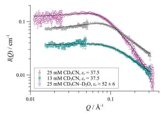
Fig. 12 SANS data and cylinder form factor fits (including an effective Hayter-Penfold structure factor S(Q) to account for charged particles) for [1][OTf] in CD<sub>3</sub>CN at 25 °C.
