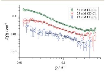
Fig. 11 SANS data and flexible cylinder form factor fits for [1][OTf] in  $CD_2Cl_2$  at 25 °C; fits are for radius 8-9 Å and lengths: 78 Å (13 mM); 156 Å (25 mM) and 332 Å (50 mM).
