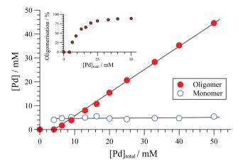
Fig. 1 Speciation of  $[(R,R)-1][BAr_F]$   $(BAr_F=B(C_6F_5)_4)$  determined by  $^{31}P\{^1H\}$  NMR  $(CD_2Cl_2,25\,^{\circ}C)$ . Solid lines through data are solely a guide to the eye. Inset shows proportion (%) of  $[Pd]_{tot}$  that is in oligomeric form.
