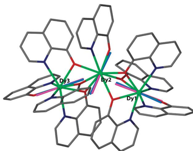
Fig. 7 Magnetic anisotropy axes for  $[\text{Dy}_3(8\text{-quinolinolate})_9]$ . Blue rods are from *ab initio* calculations, while pink rods are from electrostatic calculations. Hydrogen atoms are omitted for clarity. Reprinted with permission from ref. 23. Copyright 2014 American Chemical Society.
