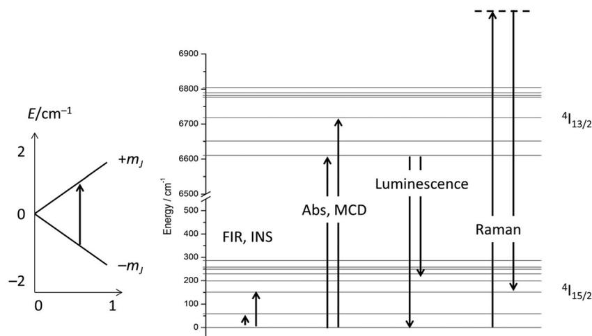
Fig. 12 Crystal field levels of ground and excited multiplets and spectroscopic techniques to study the electronic structure (example  $\text{Er}^{3+}$ ). The inset on the left depicts the splitting of the ground doublet in an applied magnetic field.
