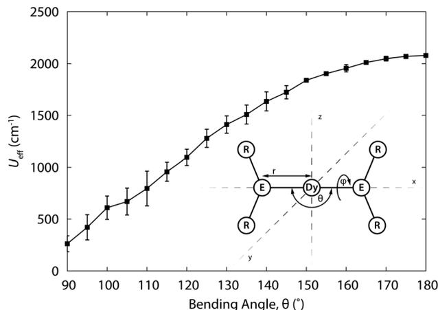
Fig. 9 Relaxation barrier  $U_{\text{eff}}$  for  $[\text{Dy}\{\text{N}(\text{SiH}_3)_2\}_2]^+$  as a function of the bending angle  $\theta$ , averaged for all torsion angles  $\phi$ . Structure of the model complex. Adapted with permission from ref. 21. Copyright 2015 American Chemical Society.
