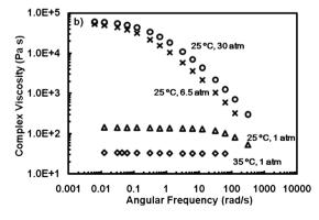
Fig. 4 Mark-Houwink plot (a) and complex viscosity curve (b) of polymers produced at different polymerization conditions with 5. Reproduced from ref. 33a with permission from the American Chemical Society.
