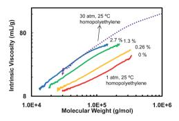
Fig. 2 Effect of ring incorporation, with the use of 16 as the latent cyclic comonomer, on topology at the polymerization condition of 1 atm and 25 °C with catalyst 5. The percentages shown are the ring contents. Reproduced from ref. 35 with permission from the American Chemical Society.
