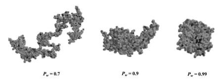
Fig. 1 Simulated conformations of polyethylene molecules formed at different chain walking possibilities. Pw refers to the probability of chain walking that controls the competition between chain-walking and monomer insertion. Reproduced from ref. 29 with permission from Wiley-VCH.
