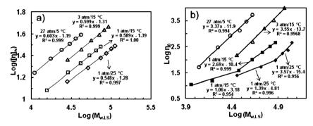
Fig. 5 Intrinsic viscosity curves (a) and complex viscosity curves (b) of narrow-distributed HBPEs of various molecular weights synthesized *via* "living" polymerization with catalyst 5. Reproduced from ref. 27f with permission from the American Chemical Society.
