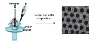
**Fig. 1** Basic "breath figures" casting technique for the formation of honeycomb structured porous polymer membranes (left). Microscopy image of a typical honeycomb structured porous film (right).
