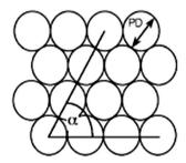
Fig. 8 The ideal hexagonal arrangement in the pores of a honeycomb structured porous film where alpha is the angle among three adjacent pores and PD is the pore diameter. Reprinted from S. D. Angus and T. P. Davis, Polymer surface design and infomatics: facile microscopy/image analysis techniques for self-organizing microporous polymer film characterization, Langmuir, 2002, 18, 9547-9553.
