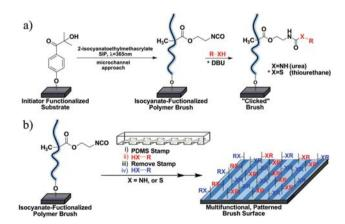
Fig. 1 (a) Schematic procedure for surface-initiated photopolymerization of 2-isocyanatoethyl methacrylate and subsequent X-isocyanate functionalization (X = thiol or amine). (b) Schematic procedure for patterning NCO-containing polymer brush surfaces with sequential X-isocyanate reactions.
