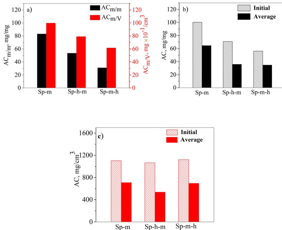
**Fig. 4** For the selectivity experiment, (a) the adsorption capacities  $AC_{m/m}$  and  $AC_{m/V}$  of the sponges for the 1st cycle of the adsorption, (b) the gravimetric/gravimetric adsorption capacities for the 1st cycle (initial  $AC_{m/m}$ ) and for the repeatability experiment of 15 cycles (average  $AC_{m/m}$ ), (c) the gravimetric/volumetric adsorption capacities for the 1st cycle (initial  $AC_{m/V}$ ) and for the 15 cycles (average  $AC_{m/V}$ ).
