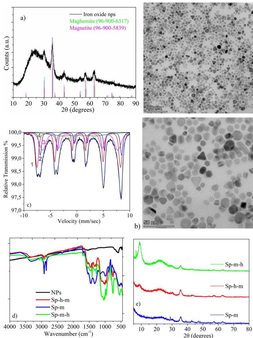
**Fig. 1** (a) The XRD pattern, (b) TEM images, and (c) the Mössbauer spectrum of the iron oxide NPs (non-stoichiometric magnetite), (d) the FT-IR spectra of all the evaluated materials (non-stoichiometric magnetite NPs and the modified sponges), and (e) the XRD patterns of the three modified sponges.
