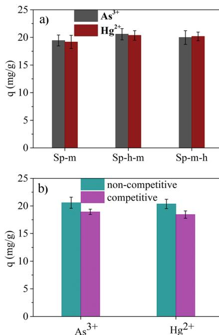
Fig. 6 (a) The adsorbed quantities of  $\text{As}^{3+}$  and  $\text{Hg}^{2+}$  in  $\text{mg g}^{-1}$  of Sp-m, Sp-h-m and Sp-m-h sponges in the experiments of single metal ion solutions and (b) the adsorbed  $\text{As}^{3+}$  and  $\text{Hg}^{2+}$  on the Sp-h-m sponge in the experiment of competitive adsorption.
