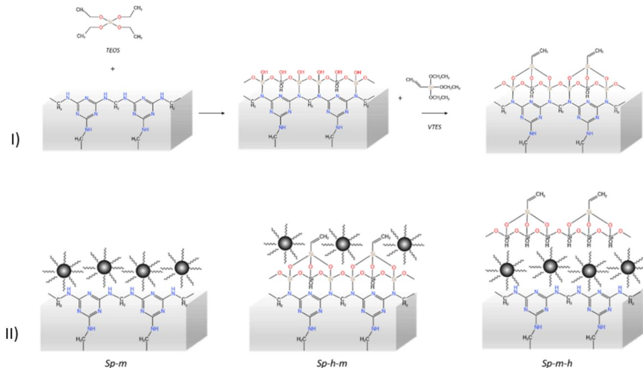
**Scheme 1** Illustration of (I) the sol-gel process for the synthesis of hydrophobic coating and (II) the functionalized (the representations of the ligands with curved lines) magnetic nanoparticles (black spheres) in either the pristine sponge or the organophilic sponges.
