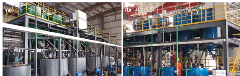
Fig. 8 Carbon dross flotation production line. (a) A 6 kt a -1 treatment line in Henan, China and (b) a 20 kt a -1 treatment line in Liaoning, China.
