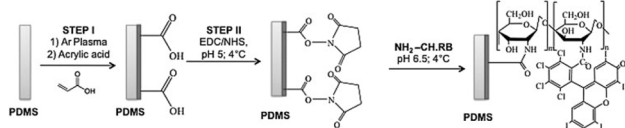
Fig. 4 Schematic illustration of the different steps for PDMS surface modification with CH. RB. Reprinted from ref. 129 Copyright (2013), with permission from Elsevier.
