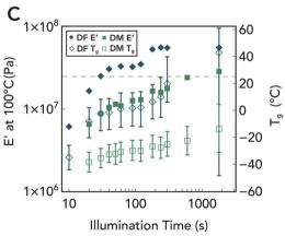
**Fig. 8** (A) DMA traces of DM network polymers illuminated for 30 s, 60 s, and 1800 s. (B) DMA traces of DF network polymers illuminated for 10 s, 60 s, and 1800 s. (C) E' at 100 °C and  $T_{\rm g}$  of DF and DM with error bars representing full width at half maximum of the glass transition. Collectively, these results suggest an increase in crosslinking density and network heterogeneity with continued light exposure.
