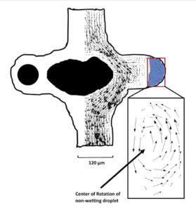
Fig. 6 Velocity fields obtained by micro-PIV in both invading wetting and trapped non-wetting phases. Reproduced from Heshmati and Piri<sup>97</sup> with permission from Elsevier, copyright 2018.
