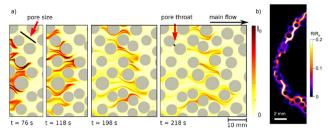
Fig. 9 a) Field of light intensity produced by cheminoluminescent reactions between reactants, reproduced from de Anna et al. 111 with permission from American Chemical Society, copyright 2014. b) Reaction rate fields for reactive transport experiment in a porous medium. The reaction rate is normalized by the reaction rate at which the image is saturated (the upper limit of the detection range). Reproduced from Izumoto et al. 112 with permission from John Wiley and Sons, copyright 2023.
