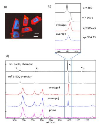
Fig. 11 a) Raman oscillatory zoned crystal of  $(Ba_{x_i}Sr_{1-x})SO_4$  with Sr (in red) enriched and Ba (in blue) enriched solid solution. b) and c) Raman signature of reference  $BaSO_4$  (barite) and  $SrSO_4$  (celestine) and the newly formed phases (i) and (j) with (b) zoom on the prominent sulfate band and (c) the complete spectra. Reproduced from Poonoosamy et al. <sup>116</sup> with permission from Springer Nature, copyright 2021.
