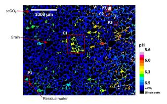
Fig. 8 Images of water pH interpreted from intensity values, scCO<sub>2</sub>, and solid grains for 8455 pore volume of injected scCO2. The flow direction is from left to right. Reproduced from Chang et al. 18 with permission from Elsevier, copyright 2017.
