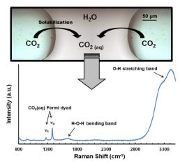
Fig. 12 Optical image of a CO<sub>2</sub>-water flow inside a microchannel and corresponding confocal Raman spectra within a water slug containing dissolved CO<sub>2</sub>. Reproduced from Liu et al. 117 with permission from Elsevier, copyright 2012.
