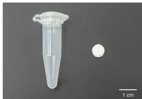
Fig. 7 Comparison of storage space requirements for a 1.5 mL microcentrifuge tube for liquid urine and a dried urine spot.
