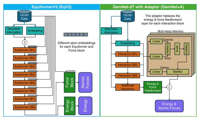
Fig. 2 Architectures of the two graph neural network models, pre-trained using the OC20 dataset for thermal catalysis.<sup>28</sup> The left is the EquiformerV2 architecture with eight Equiformer blocks. 40 The right is the GemNet-dT architecture 39 with a multi-head attention adaptor for improved transfer learning.<sup>32</sup> The number of additional interaction blocks is set to one.
