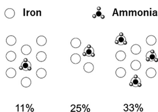
Fig. 2 Schematic presentation of ammonia coverage on Fe 110 surface.
