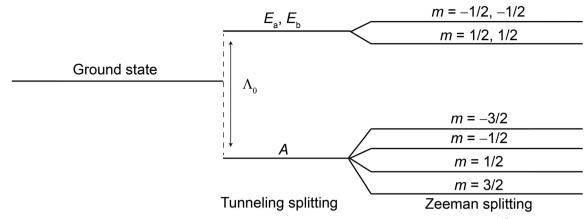
Scheme 1 Spin-states ground state energy level scheme for an isolated CF<sub>3</sub> group (without including the coupling to the <sup>13</sup>C spin, adapted from ref. 38). The energy difference between the A and  $E_a$ ,  $E_b$  manifolds is the tunneling splitting  $\Lambda_0$ .
