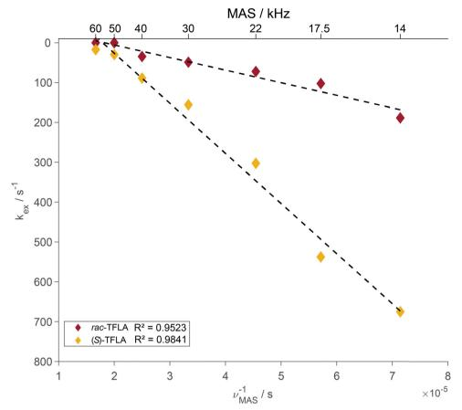
Fig. 4 Plot of the dependence of the fitted  $k_{\rm ex}$ -values (obtained from 1D nonlinear least-square fits of the experimental and simulated spectra) on the inverse of the MAS frequency,  $\nu_{MAS}$ . The corresponding value of MAS frequency is reported on the x-axis on top for each datapoint. Dashed lines are the linear regressions of the datapoints for both enantiopure and racemic TFLA samples. The  $R^2$ -values resulting from the linear regressions are reported in the leaend
