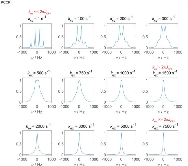
Simulation of the <sup>13</sup>C NMR spectrum of a CF<sub>3</sub> group affected by <sup>19</sup>F SD assuming a <sup>19</sup>F-<sup>13</sup>C J-coupling constant of 280 Hz and a linewidth of 10 Hz (FWHM =  $1/(\pi T_2)$ ). The spectra have been simulated as a function of the SD rate constant  $k_{\rm ex}$
