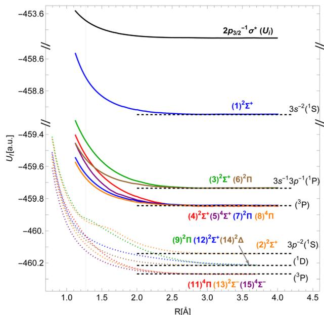
Fig. 2 Potential energy curves of the  $2p_{3/2}^{-1}\sigma^*$  state in HCl (black) and of the  $v^{-1}v'^{-1}\sigma^*$  states of the  $\text{HCl}^+$  molecular ion (colors; dotted curves taken from Pradhan *et al.*<sup>29</sup>). Horizontal dashed lines denote the energies of the  $\text{Cl}^+$  ionic states. The vertical line shows the equilibrium inter-nuclear distance of HCl.
