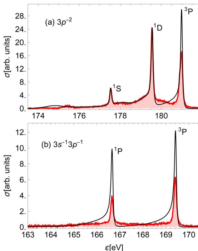
Fig. 7 Comparison of the (a) high-energy and (b) low-energy part of the calculated Auger electron spectrum (black) to the experimental result on HCl<sup>51</sup> (red). The calculated peaks were moved horizontally to match the corresponding experimental peaks and scaled to the (highest)  $^1\text{D}$  experimental peak. Each peak is denoted by the  $\text{Cl}^+$  final state in the dissociation limit.
