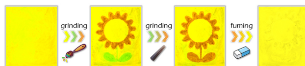
Fig. 4 Ink-free writable paper application of gold(i)-containing AIEgen 2 under 365 nm UV light.
