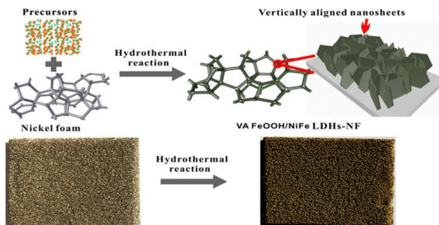
Fig. 9 Schematic illustration of the formation process of the porous VA FeOOH/NiFe LDHs-NF electrodes. Reproduced with permission from ref. 86. Copyright 2016 American Chemical Society.
