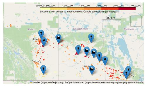
Fig. 7 Potential canola SAF production sites having access to rail, road, and population centres. The small red and yellow squares indicate canola production, the location tags with pins indicate canola crush plants and the local tags with industry symbol represents canola-biodiesel plants that use canola as a feedstock.
