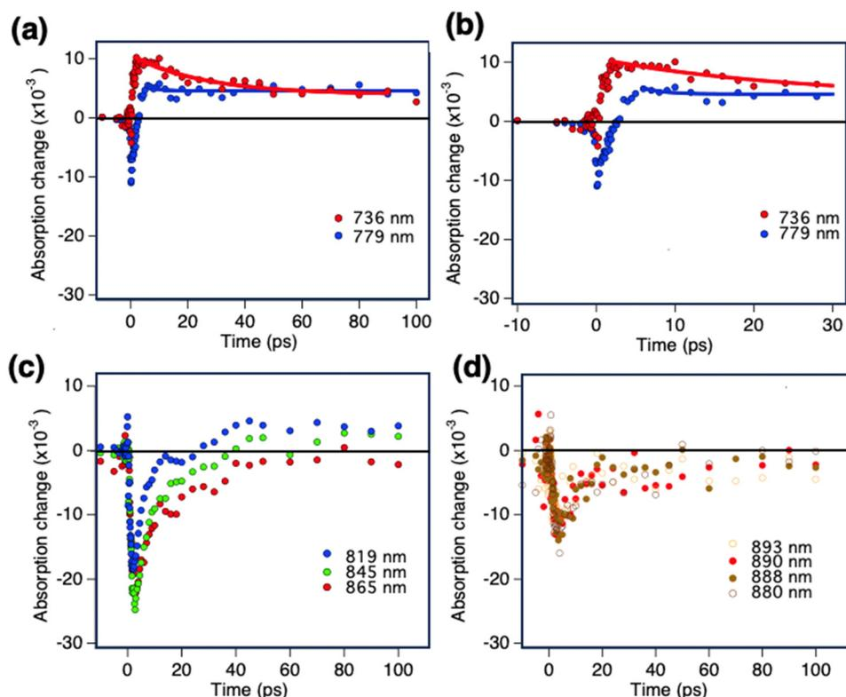
**Fig. 5** Photo-induced transient absorption kinetics for NIR-excited CZTSSe devices measured in diffuse reflectance modes. The pump wavelength was 600 nm. (a) and (b) TAS kinetics recorded in the 730–780 nm range up to 100 and 30 ps. (c) The TAS kinetics from the 800–860 nm region, and (d) the TAS kinetics further in the NIR region close to the band edge of the CZTSSe. The samples are fully functional opaque CZTSSe devices, and the experiments are performed in diffuse reflectance mode.
