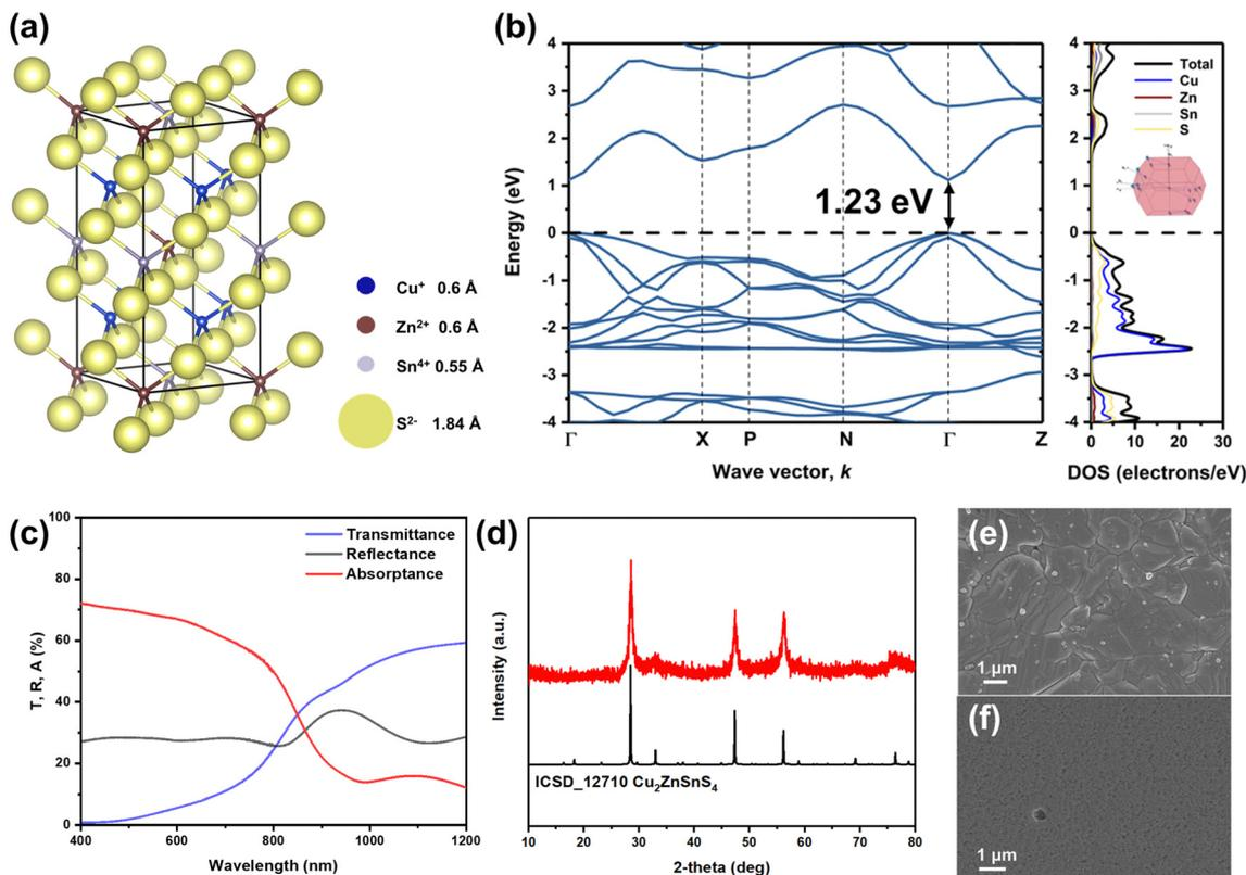
**Fig. 1** Structural, electronic, optical, and microscopic characterization of the kesterite CZTS samples. The (a) crystal structure, and (b) calculated band structure and density of states (DOS) (HSE06 hybrid function) for the kesterite CZTS. (c) Total transmittance, total reflectance, and absorbance spectra for CZTS film. (d) XRD pattern for CZTS prepared using the DMSO approach. Scanning electron microscopy images using the (e) hydrazine, and (f) DMSO synthetic approaches.
