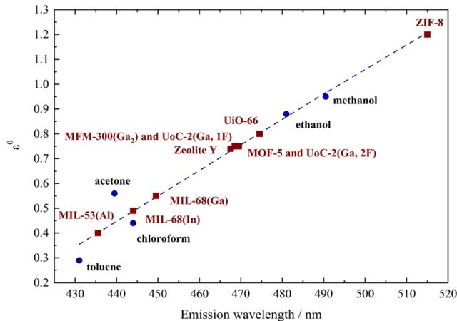
**Fig. 3** Plot of the emission maxima of Phth dissolved in different solvents (blue dots) versus the elution power  $\epsilon^0$  on alumina taken from Snyder<sup>30</sup> connected by a linear fit (blue dotted line), classifying the polarity of the respective MOFs and porous materials (red squares).
