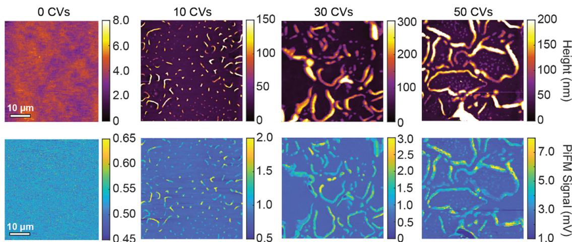
Fig. 4 AFM topography and PiFM images of a RRa P3HT thin film upon increasing numbers of CVs performed in aqueous 100 mM KTFSI after a 40 s  $-0.5$  V (*vs.* Ag/AgCl) dedoping step. 50 × 50 μm AFM topography and PiFM images are collected of an undoped RRa P3HT thin film, as well as RRa P3HT thin films that underwent 0, 10, 30, and 50 CVs.
