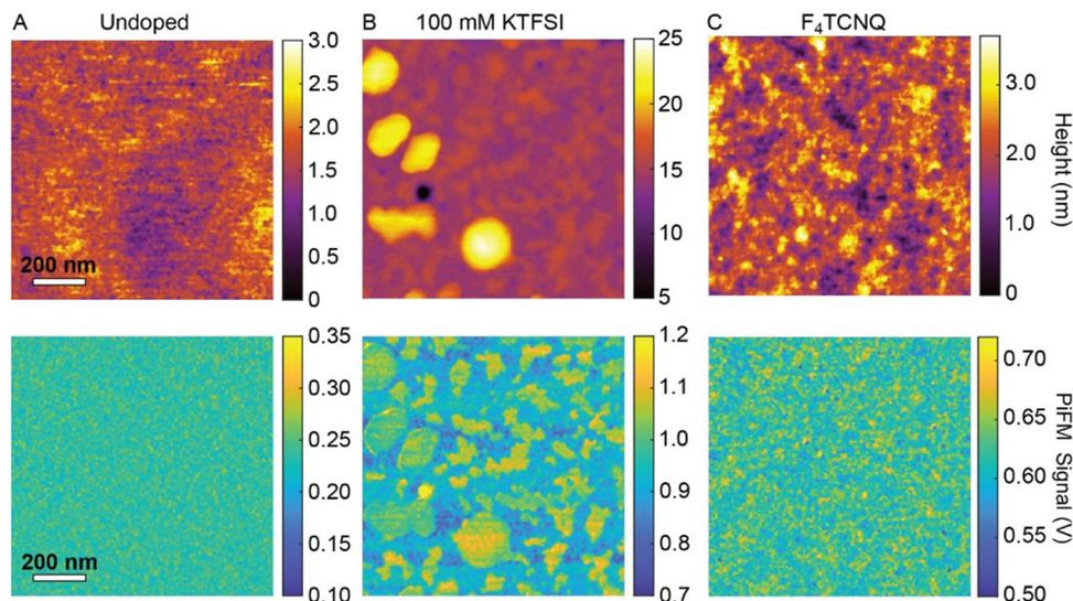
Fig. 2 PiFM images of RRa P3HT films that underwent electrochemical and chemical doping. AFM topography and PiFM nanoscale infrared images of (A) an undoped RRa P3HT film, (B) a RRa P3HT thin film doped for 20 min in an aqueous 100 mM KTFSI electrolyte, and (C) a RRa P3HT film doped in a F<sub>4</sub>TCNQ solution for 20 min.
