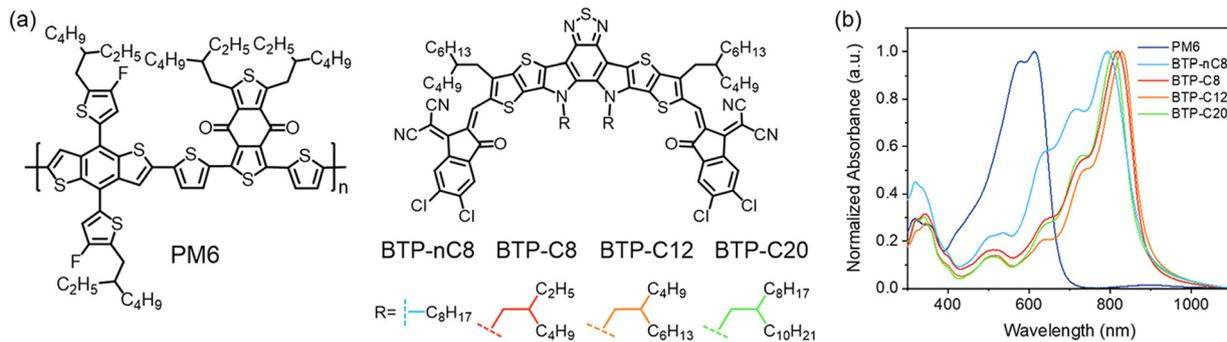
Fig. 1 (a) Molecular structures of PM6 and the FREAs. (b) Normalized absorption spectra of PM6 and FREA neat films.
