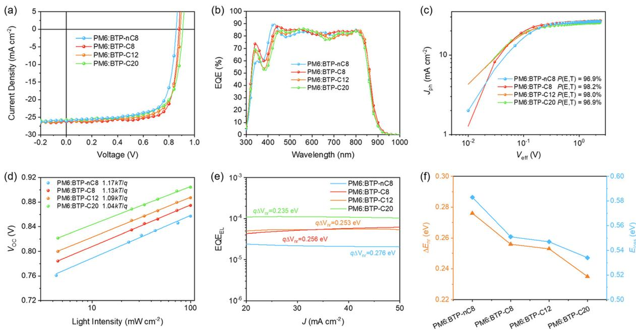
Fig. 3 (a)  $J$ - $V$  curves and (b) EQE spectra of the optimized PM6:FREA based OSCs. (c) Photocurrent density versus effective voltage curves of the PM6:FREA based OSCs. (d) Dependence of  $V_{OC}$  on the incident light intensity of the PM6:FREA based devices. (e) EQE<sub>EL</sub> curves of the PM6:FREA based devices. (f) Comparison of  $\Delta E_{nr}$  and  $E_{loss}$  of the PM6:FREA based OSCs.
