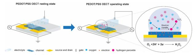
Fig. 1 A schematics of PEDOT:PSS OECT in its resting state and upon  $V_g$  operation, showing electron transfer from the polymer channel to the electrolyte and consequent generation of  $H_2O_2$ .
