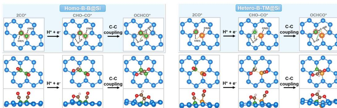
**Scheme 1** Proposed scenarios of C–C coupling mechanism on B–X@Si (homogeneous B–B@Si and heterogeneous B–TM@Si). Taking the coupling process on B–B@Si and B–Cu@Si for examples with both top and side views of corresponding optimized intermediate geometries. Dark gray and red circles symbolize ‘stabilize’ and ‘mobilize’ functions of active sites. Green narrow displays C–C bond and orange dashed line indicates the TM involvement.
