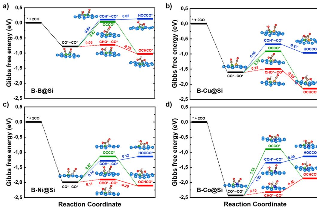
Fig. 3 Free energy profiles of different C–C coupling paths on (a) B–B@Si, (b) B–Cu@Si, (c) B–Ni@Si and (d) B–Co@Si at 0 V (vs. RHE). Inserts display the corresponding optimized structures of reaction intermediates and numbers show the corresponding reaction free energy change. The solid lines indicate the C–C coupling step. Color code: B – green, Cu – orange, Ni – silver, Co – dark blue, Si – light blue, C – brown, O – red and H – light pink.
