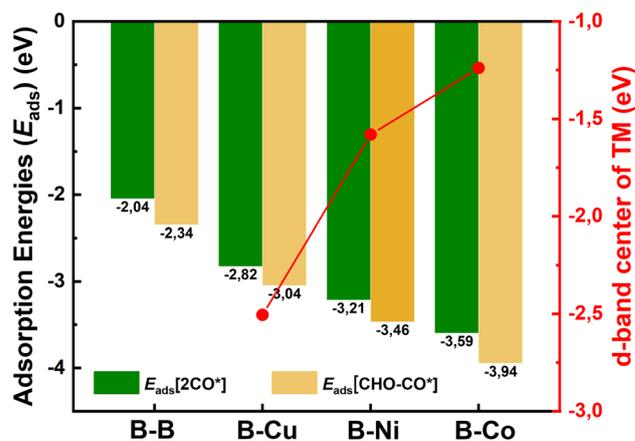
Fig. 6 Adsorption energies ( $E_{\text{ads}}$ ) of  $2\text{CO}^*$  and  $\text{CHO}-\text{CO}^*$  species on B-B@Si, B-Cu@Si, B-Ni@Si and B-Co@Si; and d-band centers of TM in bare hetero-B-TM@Si structures.
