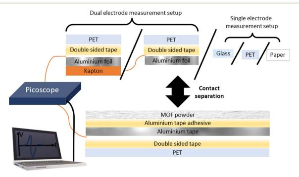
Fig. 1 Schematic of the experimental setup used for the triboelectric voltage output measurements, depicting the tape-supported MOF setup and counter material measurement modes for the dual- and single-electrode mode of measurements.
