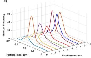
Fig. 9 a) Pressure profile of reaction system, b) HR-TEM images of MSPs (average size 490  $\pm$  9 nm), and c) particle size distribution obtained at each residence time cycle (mean residence time is 20 min and the numbers on the axis indicate multiples of mean residence time) using slug flow at  $T_G$  = 55 °C, 25% N<sub>2</sub> flow rate, and 0.0045 M
