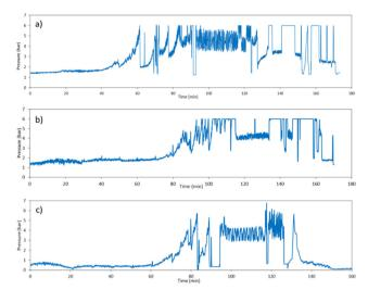
Fig. 5 Pressure profiles at the inlet of the reactor for different situations: (a)  $T_N$  = 35 °C,  $T_G$  = 55 °C, 0.0045 M NaOH, no intermediate pulsation, (b)  $T_{\rm N}$  = 55 °C,  $T_{\rm G}$  = 55 °C, 0.0045 M NaOH, 5 s pulse of methanol at 88 ml min<sup>-1</sup> flow rate, and (c)  $T_N = 35$  °C,  $T_G = 65$ °C, 0.003 M NaOH, 10 s pulse of methanol at 88 ml min<sup>-1</sup> flow rate.
