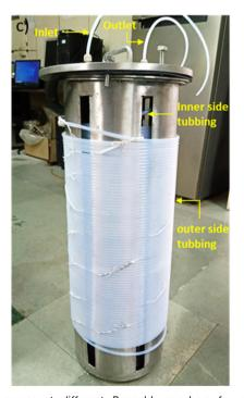
Fig. 3 a) F-curves at different Reynolds numbers for pilot-scale experiments, b)  $E(\theta)$  vs.  $\theta$  curve for the lab and pilot-scale experiments at the identical residence time, and c) photograph of the pilot-scale helically coiled tube reactor.
