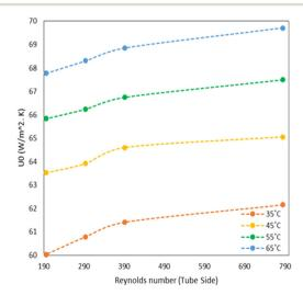
Fig. 2 Estimated heat transfer coefficient at different flow rates and temperatures.
