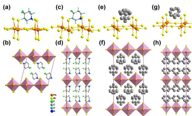
Fig. 4 Crystal structures and packing of  $[4,4\text{-DFPD}]_2\text{PbBr}_4$ .  $\alpha$  phase at 293 K along the  $b$ -axis (a and b);  $\delta$  phase at 293 K along the  $c$ -axis (c and d);  $\lambda$  phase at 420 K along the  $a$ -axis (e and f) and  $\theta$  phase at 293 K along the  $a$ -axis (g and h), respectively. All the H atoms were omitted for clarity.
