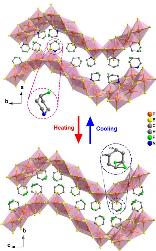
**Fig. 2** Comparison of the packing structures of  $[\text{4-FPD}]_6\text{Pb}_5\text{Br}_{16}$  at 299 K (upper) and 440 K (lower). All the hydrogen atoms were omitted for clarity.
