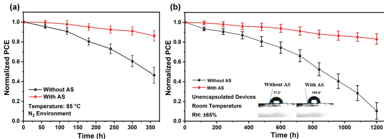
**Fig. 4** Long-term stability of PSCs prepared without and with AS method at different ambient atmosphere without any encapsulation (a) 85 °C in  $N_2$  environment; (b) 25 °C, 65%RH (the insert image showed the contact angle test of devices without and with AS method).
