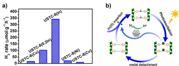
**Fig. 5** (a) Photocatalytic H<sub>2</sub> production *via* water splitting over different MOFs. (b) Proposed detachment–insertion mechanism of USTC-8(In) during the photocatalytic recycling. Reproduced from ref. 67 with permission from American Chemical Society, copyright 2018.
