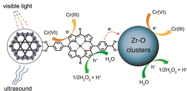
**Fig. 22** Photocatalytic reduction scheme of Cr<sup>6+</sup> to Cr<sup>3+</sup> using PCN-222 materials as catalysts throughout sonophotocatalytic processes. Reproduced from ref. 161 with permission from *American Chemical Society*, copyright 2021.
