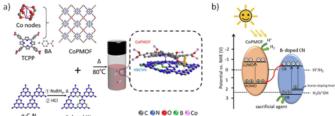
**Fig. 15** (a) Synthesis illustration of B-doped CN/Co-PMOF. (b) Proposed Z-scheme heterojunction between B-doped CN and Co-PMOF. Reproduced from ref. 85 with permission from the Elsevier, copyright 2022.
