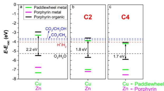
**Fig. 8** (a) Comparison between band alignments of the Cu-ZnTCPP, (b) Cu-Zn-C2 and (c) -C4 systems. The bands of metal at the paddlewheel, metal at the centre and organic atoms of porphyrins (C, N and H) are shown in green, magenta and black, respectively. The energy levels of relevant half-reactions involved in water splitting and CO<sub>2</sub> reduction to CH<sub>4</sub> and CH<sub>3</sub>OH are also shown. Reproduced from ref. 29 with permission from IOP Publishing, copyright 2021.
