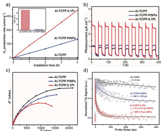
**Fig. 4** (a) Photocatalytic H<sub>2</sub> production rates of Al-TCPP, Al-TCPP-PtNPs, and Al-TCPP-0.1Pt (inset: the calculated TOFs of Al-TCPP-PtNPs and Al-TCPP-0.1Pt). (b) Photocurrent responses, (c) EIS Nyquist plots and (d) comparison of the ultrafast TA kinetics (pump at 400 nm and probe at 540 nm) for Al-TCPP, Al-TCPP-PtNPs, and Al-TCPP-0.1Pt. Reproduced from ref. 66 with permission from Wiley-VCH, copyright 2018.
