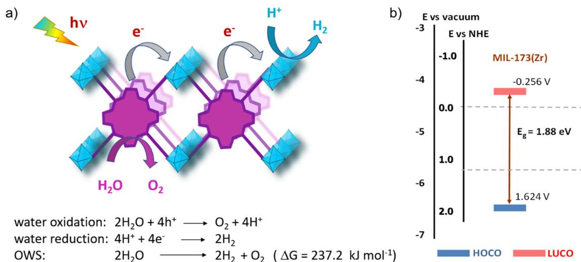
**Fig. 3** General mechanism of photoinduced charge separation in MOFs triggered by light absorption and photoinduced charge transfer to the near metal node with the associated half and overall water splitting reactions equations (a), and energy level diagram for the PMOF MIL-173(Zr) (b).
