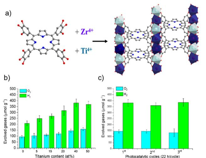
**Fig. 17** (a) Synthesis scheme for the mixed metal MIL-173(Ti/Zr), (b) photocatalytic OWS under simulated sunlight irradiation using MIL-173(Zr) and MIL-173(Ti/Zr) solids having different Ti at% contents, and (c) photocatalytic stability upon 3 cycles. Reproduced from ref. 109 with permission from the Royal Society of Chemistry, copyright 2022.
