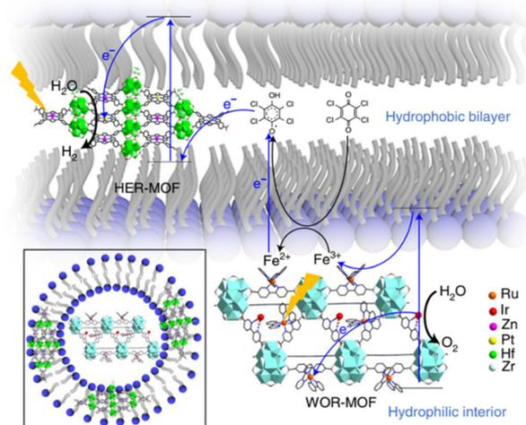
**Fig. 16** Structure of the liposome-MOF for OWS and the proposed 'Z-scheme' electron-transfer chain in the liposome-MOF system. Reproduced from ref. 53 with permission from Springer Nature, copyright 2021.
