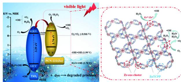
**Fig. 19** Schematic diagram of the possible visible-light-driven photocatalytic degradation mechanism toward the TP-222(Zn) composite with the integration of TiO<sub>2</sub> NPs into PCN-222(Zn). Reproduced from ref. 121 with permission from the Royal Society of Chemistry, copyright 2017.
