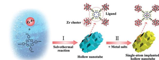
**Fig. 11** Synthesis scheme of the hollow nanotube MOFs and immobilization of single-atom within hollow nanotube MOFs. Reproduced from ref. 76 with permission from Wiley-VCH, copyright 2018.
