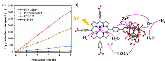
**Fig. 9** (a) Photocatalytic H<sub>2</sub> production rates of PtTCPP, PCN-222, PtNPs/PCN-222, and PCN-222(Pt). (b) Proposed photocatalytic mechanism of dual catalytic centres in PCN-222(Pt). Reproduced from ref. 70 with permission from the Elsevier, copyright 2022.
