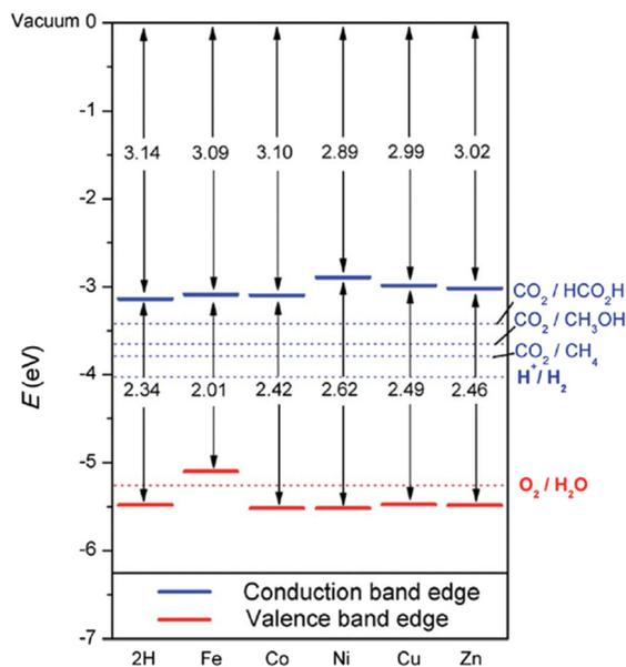
**Fig. 6** Bandgaps and band edge positions with respect to the vacuum level, as calculated with the HSE06 functional. Energy levels corresponding to redox potentials of water splitting and carbon dioxide reduction reactions producing methane, methanol, and formic acid at pH 7 are also shown with dotted lines. Reproduced from ref. 27 with permission from the Royal Society of Chemistry, copyright 2015.
